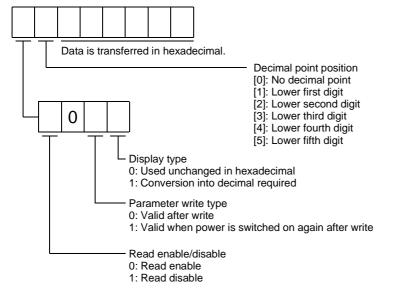
Enable/disable information changes according to the setting of parameter No.19 "parameter write inhibit". When the enable/disable setting is read disable, ignore the parameter data part and process it as unreadable.
